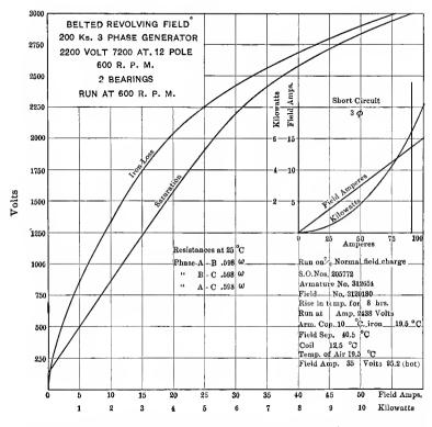
FIG. 86. Characteristic curves of 200 k.w., three-phase alternator (Westinghouse).
